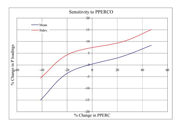
Phosphorous loadings are sensitive to PPERCO as can be seen from the Figure above. A 20% decrease in the value of PPERCO caused a 15 % decrease in P loadings. The relationship between POSKD and P loadings is more complex as can be seen from the Figure below. The P loadings behave in a non-linear manner with changes in POSKD.
