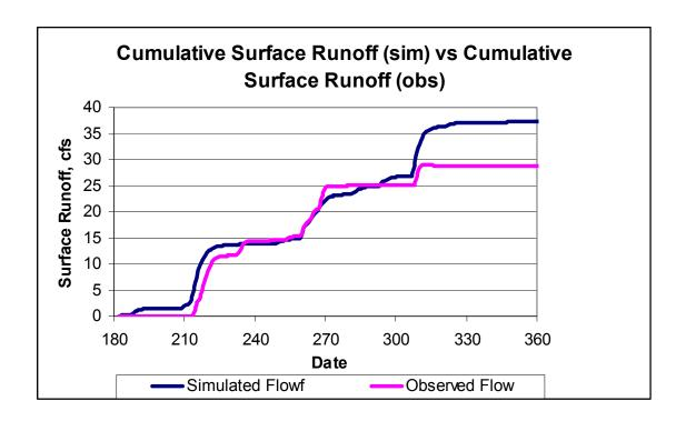
Although SWAT2000 did not predict every single runoff event precisely, the cumulative results appear to be relatively close. Cumulative surface runoff is slightly over predicted by SWAT. The general shape of the lines follows a similar pattern.
