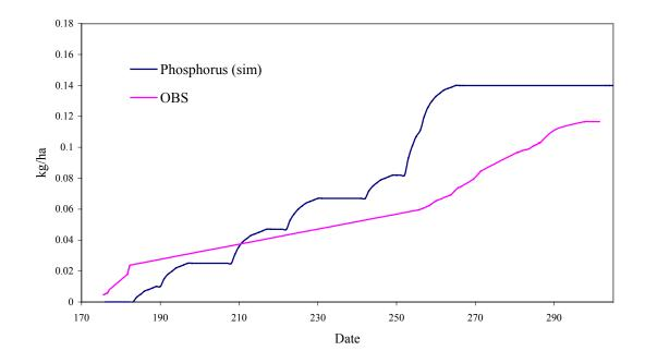
The behavior is different between the observed and the simulated. Again the apparent lack of an outflow event between day 200 and 250 contributes significantly to the differences.
