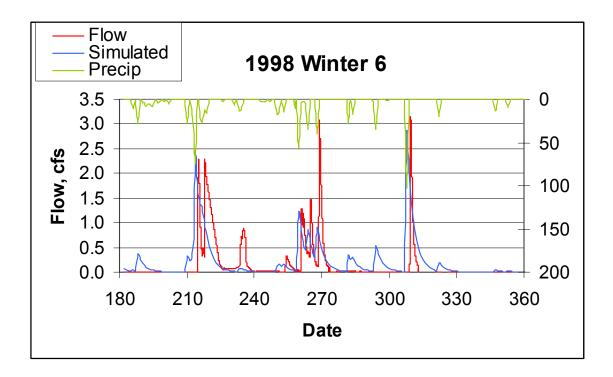
SWAT2000 predicted surface runoff relatively well. There are a couple of runoff events that were simulated that do not show on the observed data. This could be due to improper collection of the original data. As discussed in class, there are several factors
